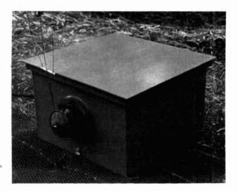
fig. 3. Coupler houses high voltage matching circuit components.
